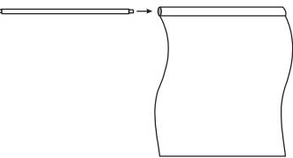
Hook release material rod on brackets located at the rear of the upper plate
